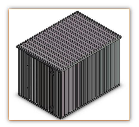
**12.** Roof is fixed with bolts from connection points inside of the cabin.
